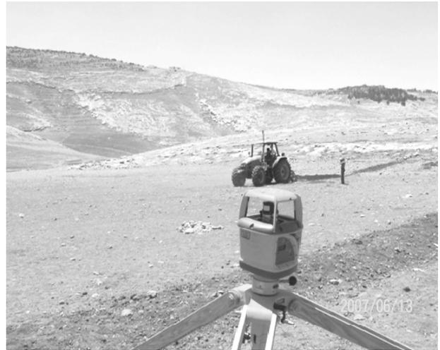
**Fig. 2** The laser beam transmitter mounted on a tripod on uphill side.
