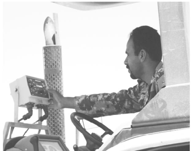
**Fig. 4** Display panel mounted in front of the tractor operator.
