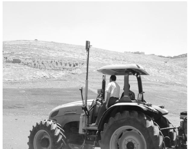
**Fig. 3** Laser receiver mounted on a telescopic mast on the tractor.
